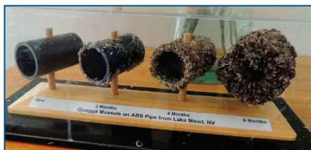
Quagga mussels in Lake Mead completely clogged a pipe in 6 months.
