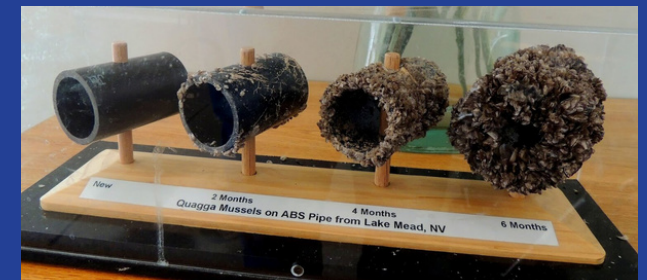
Quagga Mussels on ABS pipe from Lake Mead, NV.
